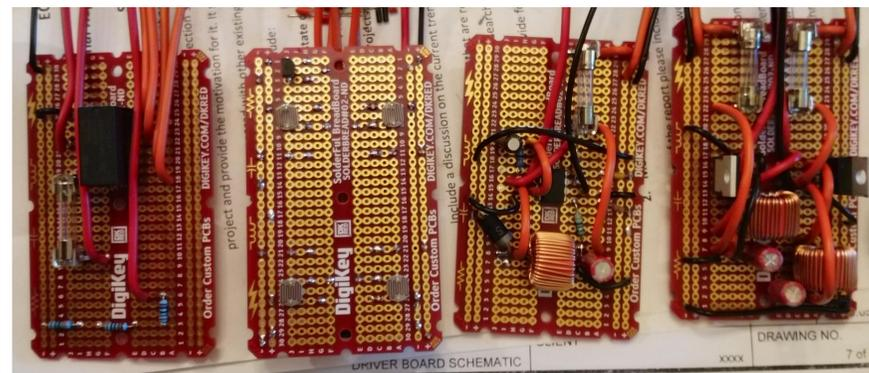
From left to right, a water pump enable relay circuit and solar panel production monitoring circuit, an LDR-based tracking circuit, a high-current variable power supply, and a simple 3.3V and 5V power supply circuits on one board. Every one of these boards is available in multiple configurations, ranging from low-power and low-cost, to high-power and high-cost, and even with some premium extra options available.
