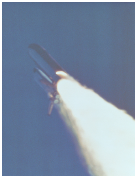
Figure 6.1: An image of the solid rocket booster leaking fuel, seconds before the explosion. By NASA (Great Images in NASA Description) [Public domain], via Wikimedia Commons
