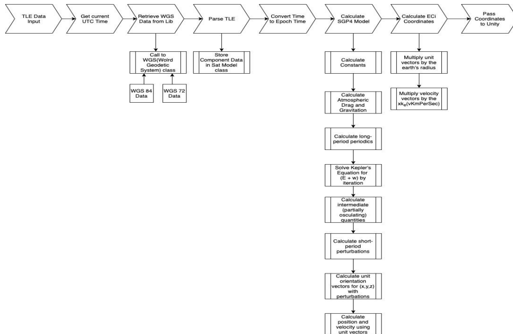
Figure 4. Flowchart of converting TLE to unit/velocity vectors.
