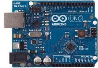
THE ARDUINO UNO IS A MICROCONTROLLER BOARD BASED ON THE ATMEGA328. IT HAS 20 DIGITAL INPUT/OUTPUT PINS (OF WHICH 6 CAN BE USED AS PWM OUTPUTS AND 6 CAN BE USED AS ANALOG INPUTS), A 16 MHz RESONATOR, A USB CONNECTION, A POWER JACK, AN IN-CIRCUIT SYSTEM PROGRAMMING (ICSP) HEADER, AND A RESET BUTTON.
