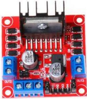
THIS MODULE WILL ALLOW YOU TO EASILY AND INDEPENDENTLY CONTROL TWO MOTORS OF UP TO 2A EACH IN BOTH DIRECTIONS.
